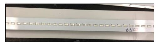
Figure 5: Thermal interface material used under LED PCB
