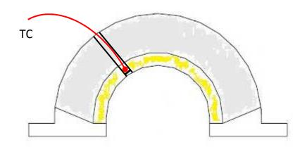
Figure 19: ChromaLit Linear thermocouple insertion
