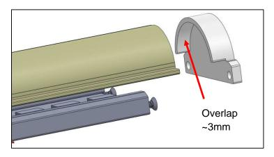
Figure 10: Example of screw on end cap with overlap
