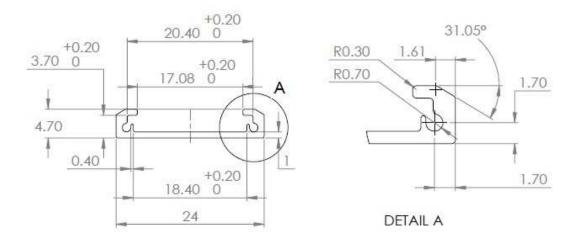
Figure 13: Aluminum extrusion slider architecture
