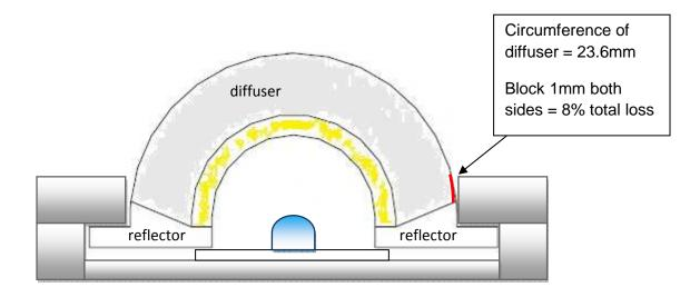
Figure 9: Housing light loss example
